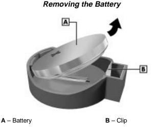
**5.** Remove the battery and discard in accordance with the manufacturer's instructions.
